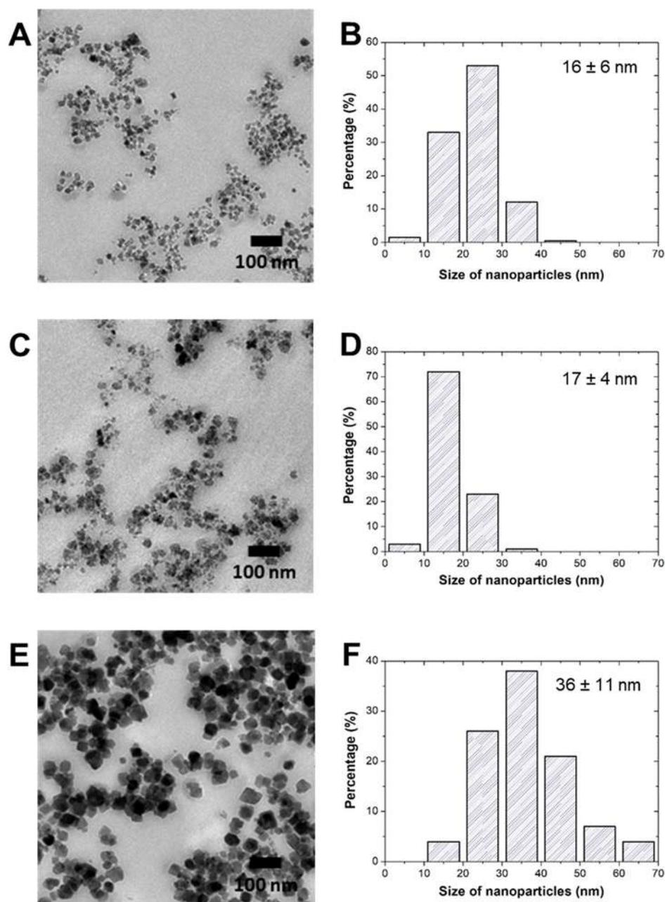
**Figure 4.** TEM images of magnetite nanoparticles obtained in different experimental conditions. (A and B) Magnetite crystals from the inorganic control experiment and size distribution; (C and D) magnetite crystals from the E66A/D70A MamC experiment and size distribution; (E and F) Magnetite crystals from the WT MamC experiment and size distribution.
